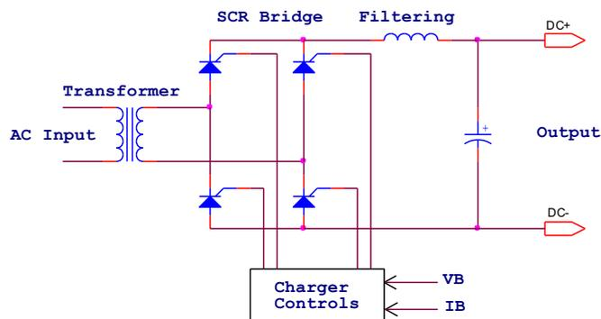
Fig. 4: SCR battery charger
