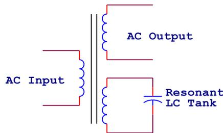
Fig. 2: Ferroresonant transformer
