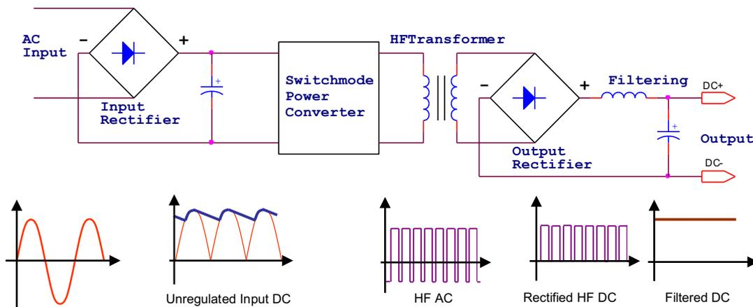
Fig.5: Typical isolated high frequency battery charger employing a high frequency transformer
