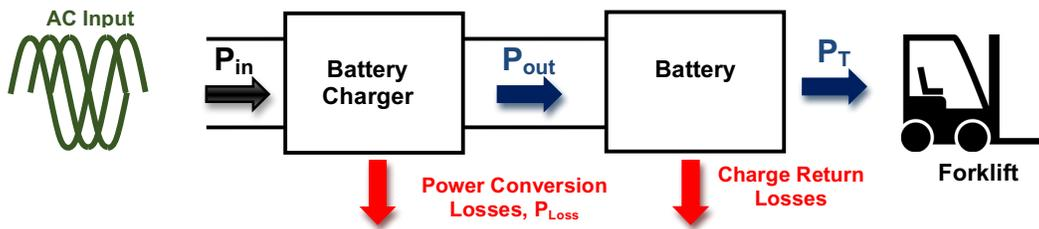
Fig. 1: Battery charger block diagram
