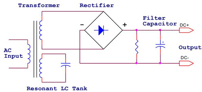
Fig. 3: Ferroresonant battery charger
