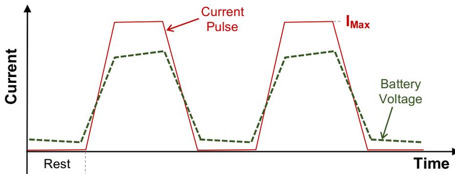
**Fig. 3: Battery voltage and current waveforms during an ionic profile phase**
