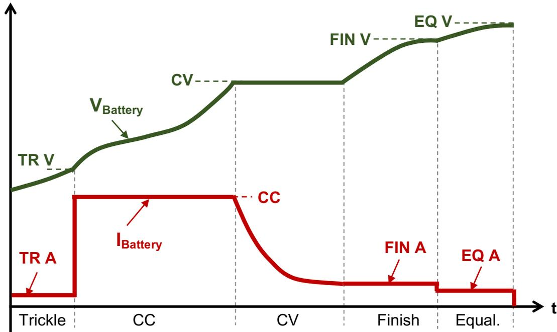
**Fig. 1: Typical charge profile for lead acid battery**
