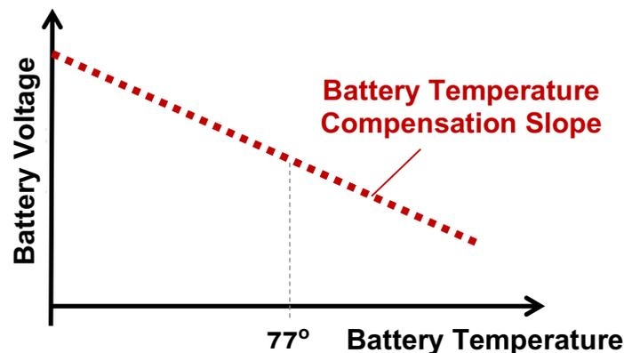
**Fig. 2: Lead acid battery voltage versus temperature**
