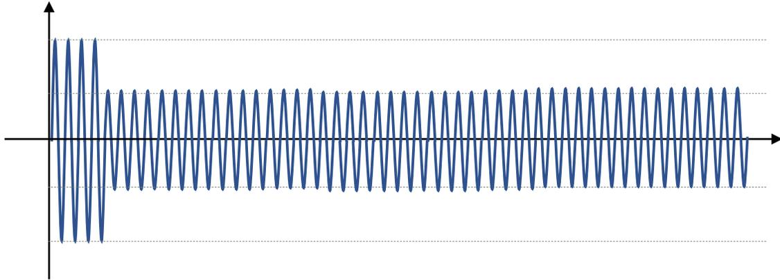
**Fig. 5: AC undervoltage**
