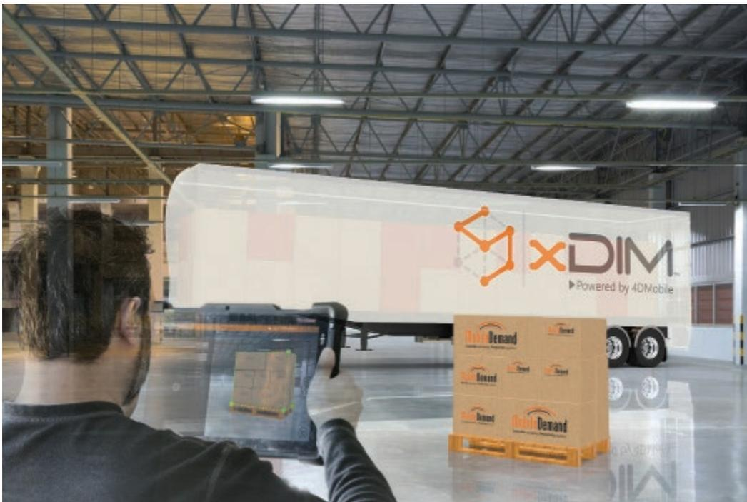
A 3-D camera on a tablet brings load dimensioning technology to the package, rather than the other way around.
