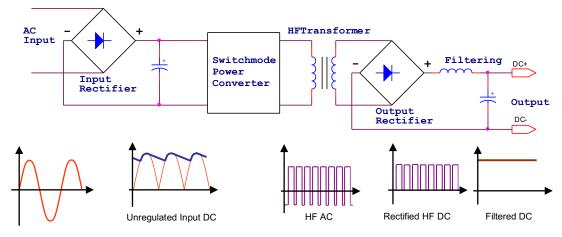
Fig. 5: Typical isolated high frequency battery charger employing a high frequency transformer
