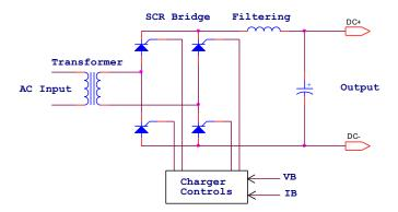
Fig. 4: SCR battery charger
