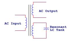
Fig. 2: Ferroresonant transformer
