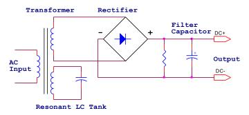
Fig. 3: Ferroresonant battery charger
