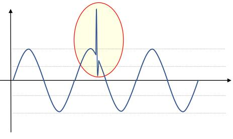
Fig. 1: Typical AC voltage spike
