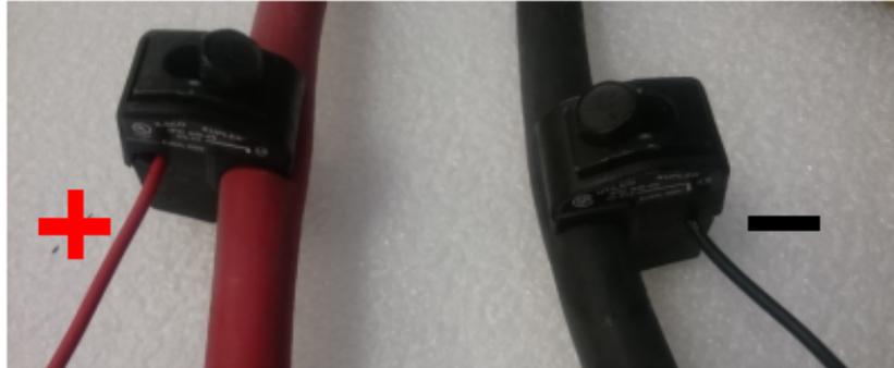
2. Once the positive lead is connected, the Battview will blink Blue one time.
