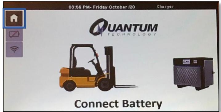
12.Ensure that the LCD on the charger is calibrated by clicking the home button and verify you can navigate the menu.
